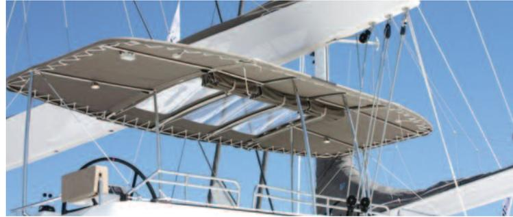
The practical application of photovoltaic fabrics has taken an important step forward with the introduction of a bimini top that not only blocks the sun, but also generates enough power to recharge on-board batteries or power small electronics. Catamaran builder Lagoon, Dickson-Constant and Nv Equipment debuted the application during the Cannes International Boat and Yacht Show this past fall aboard the 62-foot Lagoon 620.
