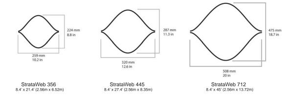
StrataWeb panels can be provided in cell heights of 3" (75mm), 4" (100mm), 6" (150mm), and 8" (200mm). Standard panels are constructed of 58 strips with the dimensions above.
