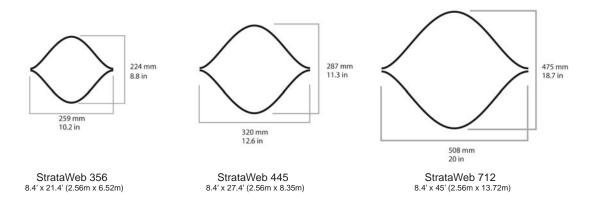
StrataWeb panels can be provided in cell heights of 3" (75mm), 4" (100mm), 6" (150mm), and 8" (200mm). Standard panels are constructed of 58 strips with the dimensions above.
