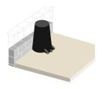
Encapsulate and stabilize the Sleeve-It unit by placing and compacting sufficient backfill material layers as required.
