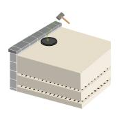
Punch the perforated lid using a mallet or hammer to expose the inside of the Sleeve-It unit. Detached lids can be left inside the unit or discarded prior to pouring of infill material.
