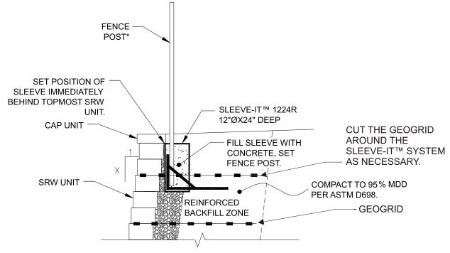
\*FENCING SYSTEMS APPROVED FOR USE WITH SLEEVE-IT™ 1224R ARE LIMITED TO THE FOLLOWING HEIGHTS: CHAIN LINK - UP TO 8-FT, ORNAMENTAL - UP TO 6-FT (WOODEN, PVC, METAL). POST SIZE 4"X4" MAX.
